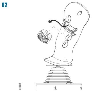
Disconnect the cable from the defective roller and connect it to the replacing part. Gently snap the roller back in place within the handle. Make sure that no wires get pinched on the inside.
