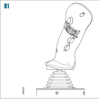
Lift the edge of the roller gently by using a thin tool. (ex. knife or screwdriver)
